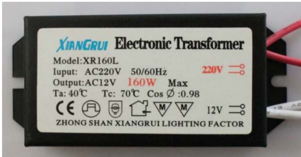
Figure 10.1. An electronic transformer
