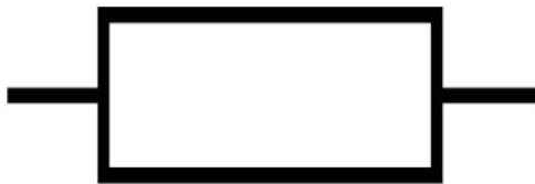
Figure 6.2. International resistor circuit symbol
