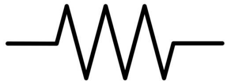
Fig.6.3. USA resistor circuit symbol
