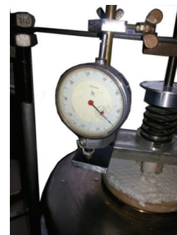
Fig. 3. Pressing device of the sintering setup
