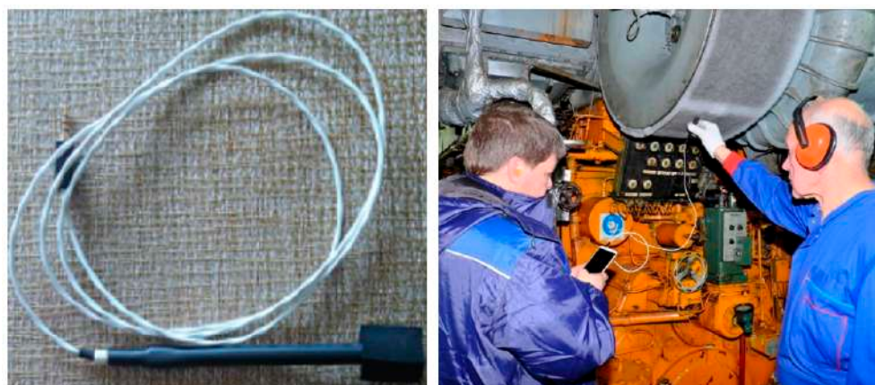
Figure 4. Recording the vibration of the turbocharger using the EM-4015-BC electret microphone.
