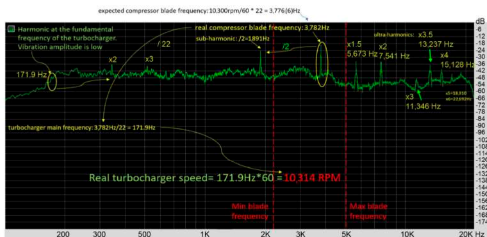
Figure 3. The acoustic signal spectrum of the TCA 66-20072 turbocharger compressor at 50% load mode of the 5S60MC engine (4500 kW, 85 rpm).
