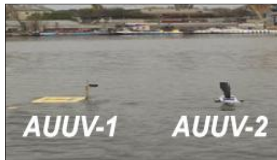
Fig. 8. Mutual arrangement of the AUUV-1 and the AUUV-2 during the experiment testing the operability of the adhesion mode
