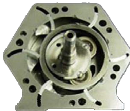
Fig. 4. Rotary air engine developed by Angelo di Pietro
