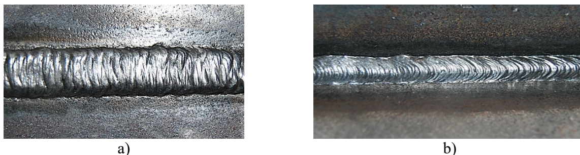
Fig. 2. Outer appearance of butt weld (a) and fillet weld (b) joints in welding positions: a) - overhead; b) – horizontal-overhead.
