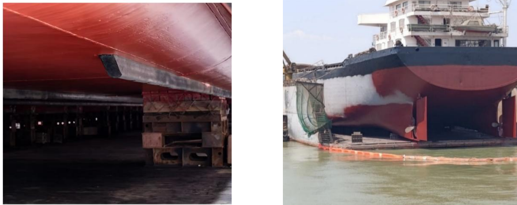
Figure 5. River–sea vessel retrofit in a floating dock
