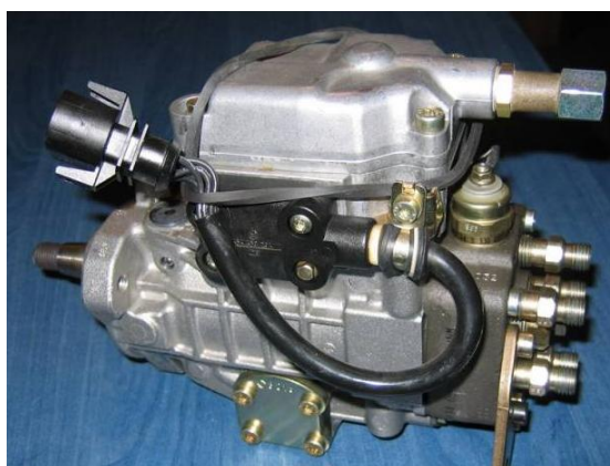
Figure 3.3 – VE type HP HPD by R. Bosch
