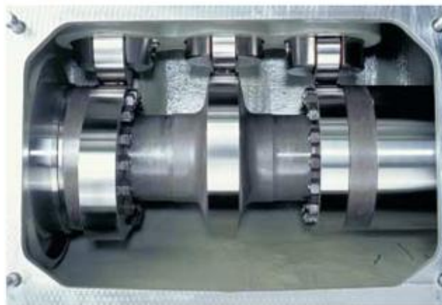
Figure 1.9 – Camshaft and valve mechanism
