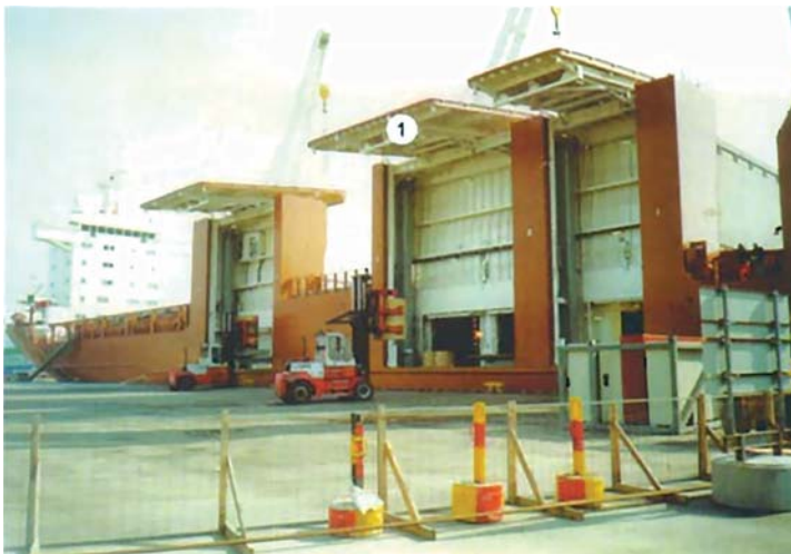
Figure 9.14 – Ship with three side doors [21]
