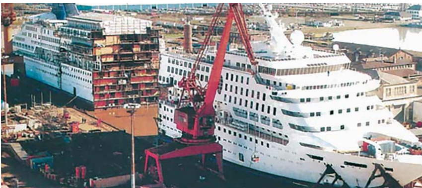
Figure 14.5 – A passenger ship is being lengthened to increase capacity [21]
