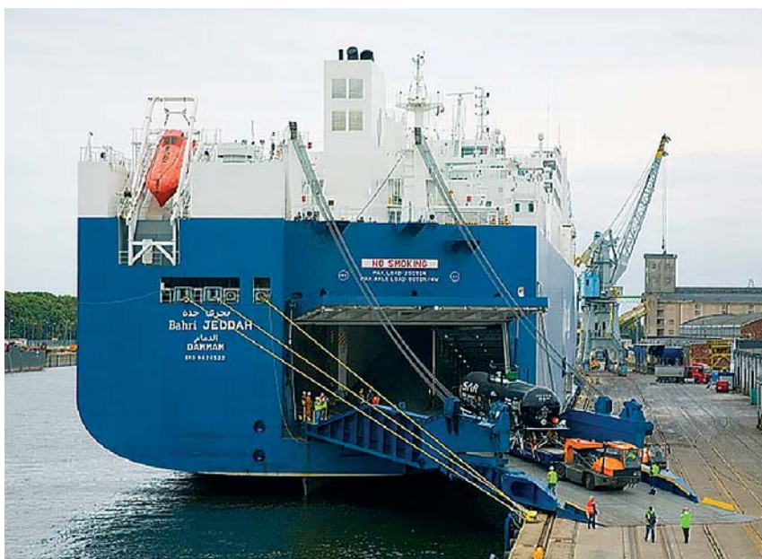
Figure 1.5 – Discharging of the Ro-Ro Ship
