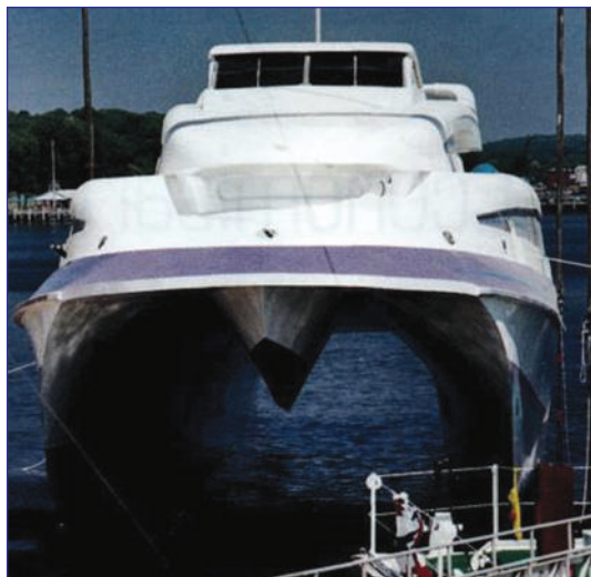
Fig. 4. Planning Catamaran with Interhull Bridge of Wedge-shaped Form and Internal Rounding Frames
