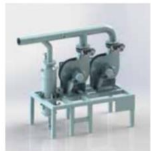
Hydro Cyclone & Blower
