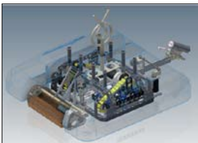
Fig. 4. Wheeled MRs with permanent magnets: a — for cleaning; b, c — for inspection
