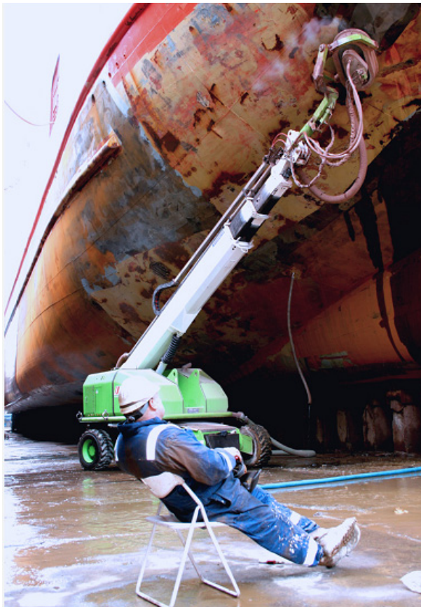
Fig. 2. Cleaning MR based on a wheeled complex with a universal CD and a telescopic lever
