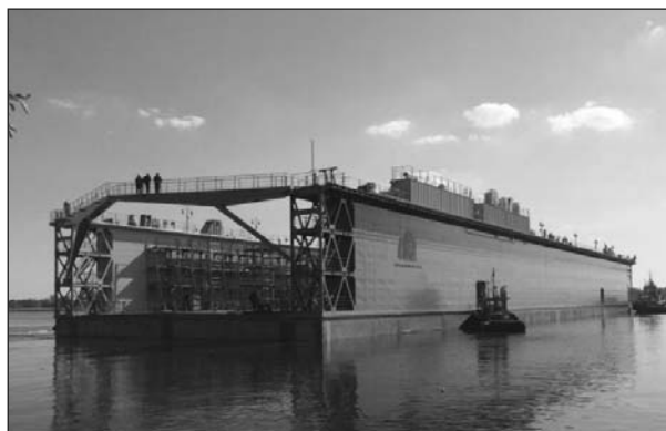
Fig. 1. Composite floating dock with the cargo capacity of 7100 tons that was built at the Kherson State Plant «Pallada».
