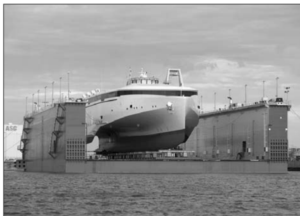
Fig. 2. Steel transport floating dock at the Australian Marine Complex (Australia)
