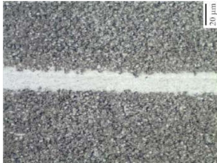
Figure 8. Microstructure of the diffusion bonded joint of nickel-plated 14Cr17Ni2 alloy at T_w = 900^\circ\text{C} ; P_w = 5\text{ MPa} ; t_w = 35\text{ min}
