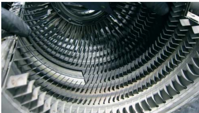
Fig. 2.18. Guide vanes of the 10-stage single-spool compressor of the T58 engine
