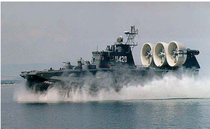
Fig. 1.3. Project 1232.2 Zubr hovercraft (Ukraine) (5 UGT 6000 engines; full displacement – 555 tons, full speed – 63 knots)
