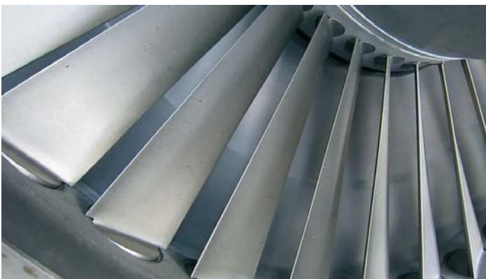
Fig. 2.25. Inlet guide vanes of the J79 engine
