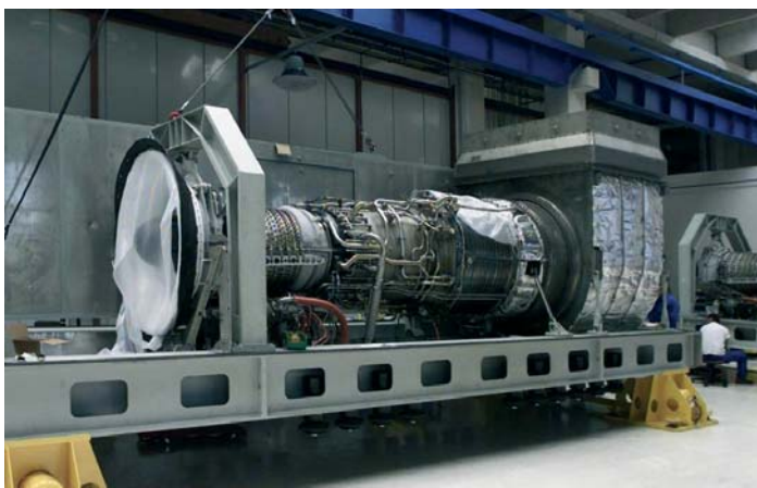
Fig. 1.8. LM2500 engine before delivery to the customer
