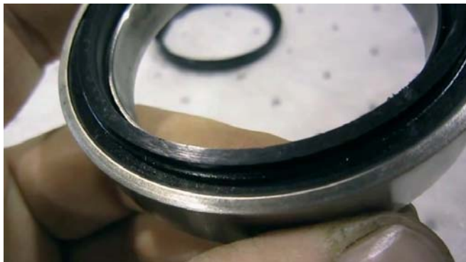
Fig. 5.29. Elements of a graphite contact seal
