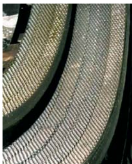
Fig. 5.11. Honeycomb inserts of labyrinth seals
