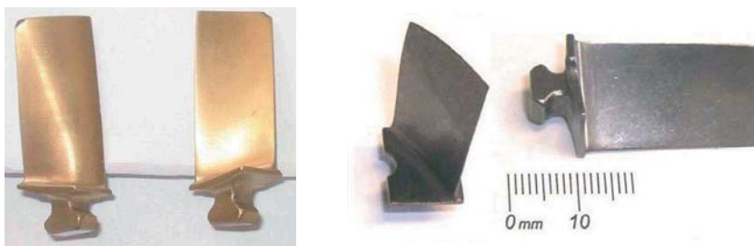
Fig. 2.7. Blades with stream-type tails
