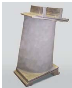
Fig. 2.30. Nozzle vane of the Turboatom GTE-45-3 engine
