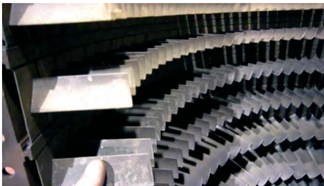
Fig. 2.17. Guide vanes of the 17-stage single-spool compressor of the J79 engine
