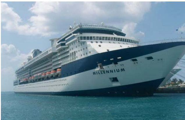
Fig. 1.5. Millennium-class cruise ship (2 LM2500+ engines with heat recovery; full displacement – 90,238 tons, speed – 21 knots, crew – 920 people, passenger capacity – 1,950 people)
