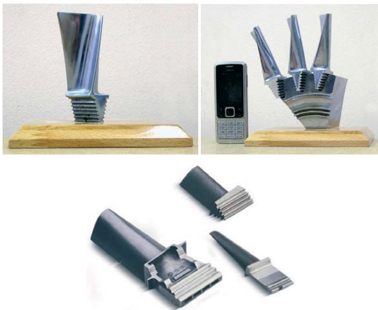
Fig. 2.45. Turbine blades with fir-tree tails
