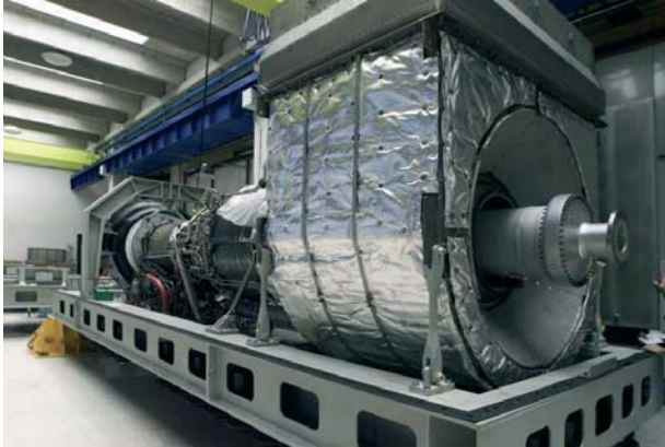
Fig. 6.43. GE Aerospace LM2500 engine with a snail-type exhaust device
