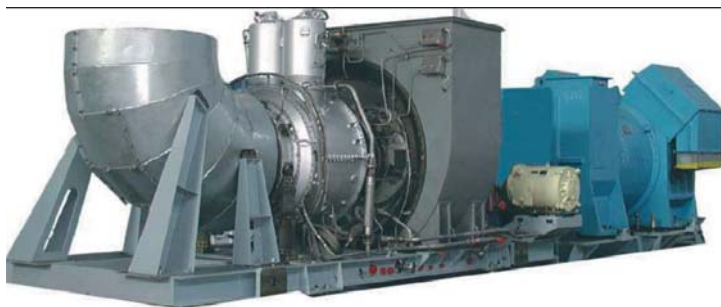
Fig. 6.44. Zorya-Mashproekt UGT2500 engine with a knee-shaped exhaust device
