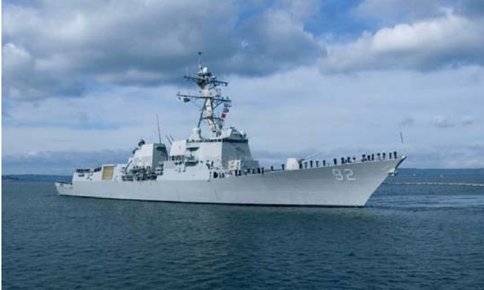
Fig. 1.2. Arleigh Burke-class guided missile destroyer (USA) (4 LM2500 engines; full displacement – 8315 tons, full speed – 30 knots)
