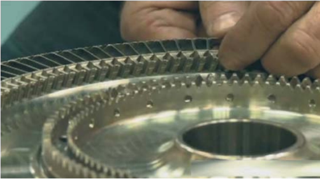
Fig. 3.12. Turbine disk with triangular end splines
