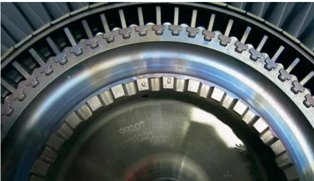
Fig. 3.13. GE Aerospace turbine disk with end curved splines
