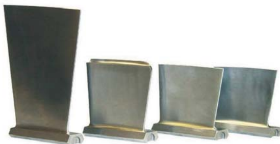
Fig. 2.12. Blades of the GTN-25 engine compressor
