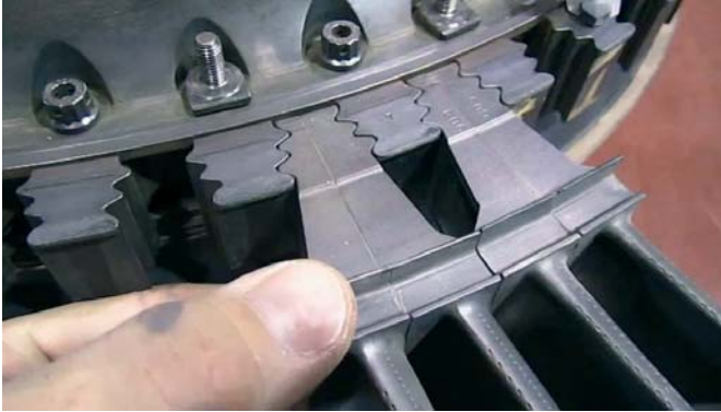
Fig. 2.44. Installing the two blades in one groove
