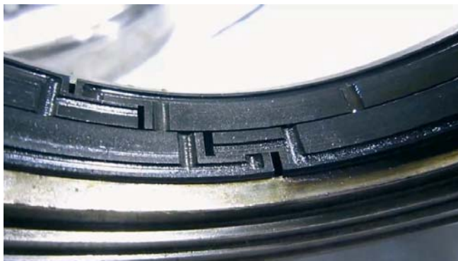
Fig. 5.30. Double-row graphite contact seal (section view of the rings)
