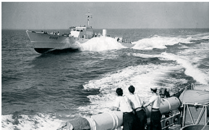
Fig. 1.1. MGB 2009 gunboat (Great Britain) (displacement – 95 tons; maximum speed – 31 knots)
