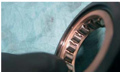
Fig. 4.8. Roller bearing with a solid bronze separator
