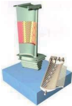
Fig. 2.50. Cooled turbine blade of the Zorya-Mashproekt UGT25000 engine, its casting core, and core box
