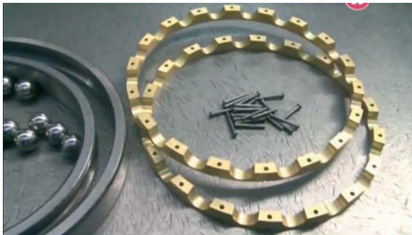
Fig. 4.6. Disassembled ball bearing with riveted separator
