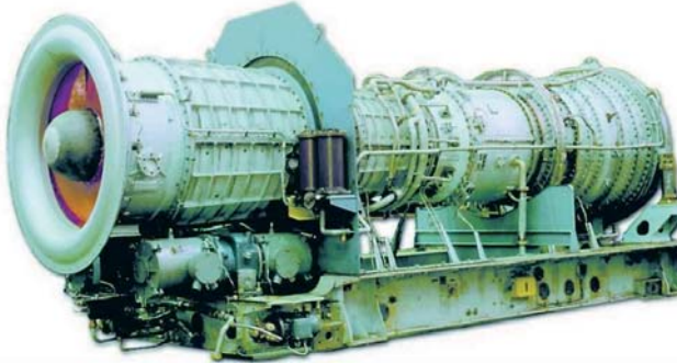
Fig. 6.2. Zorya-Mashproekt UGT16000 engine with axial-type inlet device [12]
