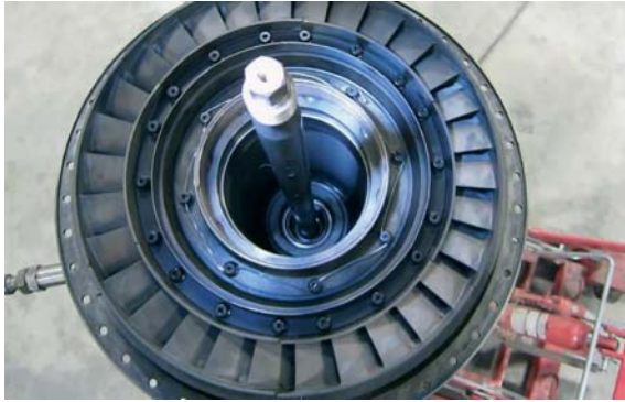
Fig. 3.9. Installing the center tie bolt on a GE Aerospace T58 engine
