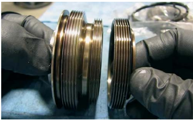
Fig. 5.24. Elements of two-tier labyrinth oil seals
