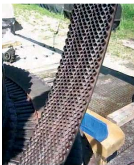
Fig. 5.11. Honeycomb inserts of labyrinth seals
