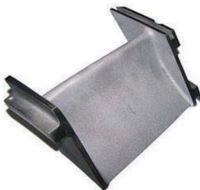
Fig. 2.29. Nozzle vane of the GTK-10-4 engine
