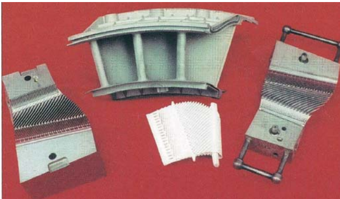
Fig. 2.32. Cooled nozzle device, its casting rod, and a device for manufacturing
