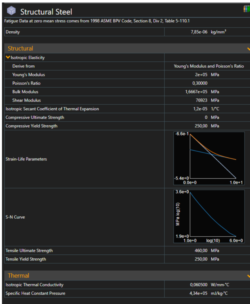
Picture 11: Properties of structural steel
